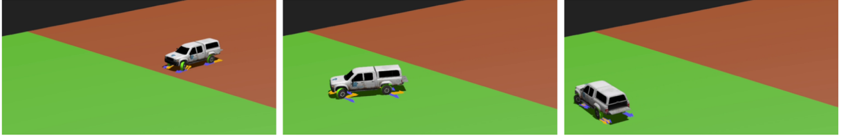
Figure 13: A moving vehicle brakes hard on a terrain with a friction texture. The region of the terrain with the orange texture has a high friction coefficient in the direction lateral to the tires. However, when the vehicle skids onto the green region, the structure direction changes suddenly and the vehicle begins to fishtail due to friction anisotropy.
