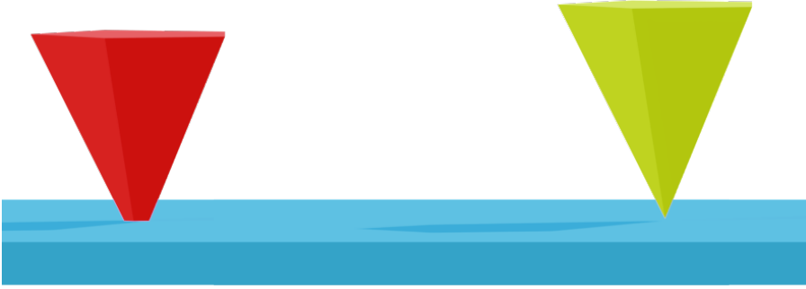
Fig. 6. Two coarse pyramids fall onto an analytical SDF box. The simulation with discrete collision detection (left) shows clear interpenetration, while our method on the right detects sharp contacts in time.
