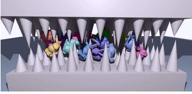
Figure 4: Bunny Iron Maiden: A group of bunnies is sandwiched between plates with spikes. All geometries are encoded by analytical (spikes and plates) and voxel-based signed distance functions (bunnies). This challenging test creates a landscape of narrow basins of attraction and disjoint contact regions.
