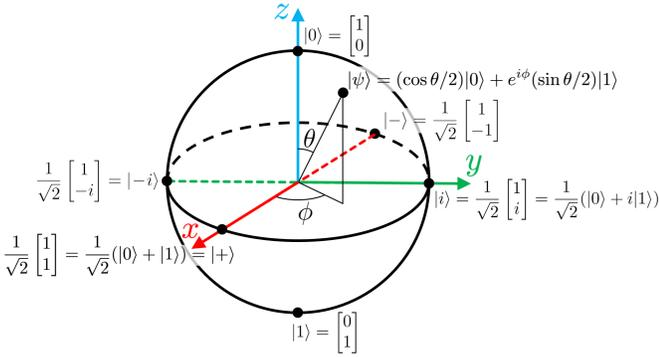
Fig. 2. The Bloch sphere’s surface contains all physically distinguishable states of a single qubit whose state can be described with a state vector  $|\psi\rangle$ . Certain states have standard names like  $|+\rangle$  and  $|i\rangle$ .
