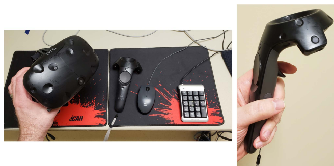
Fig. 4. The equipment for Study 1: HTC Vive headset and controller (held in the NDH), mouse (for the DH) and keypad (to advance to the next trial after a break).
