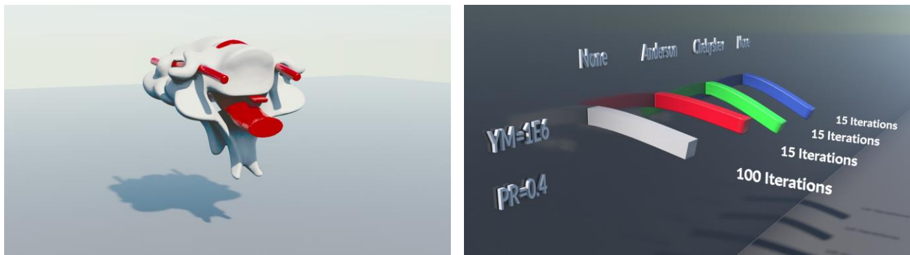
Figure 1: Real-time simulation of a spinal ligament (7k tetrahedral, left), and deformable beam (5k tetrahedral, right).
