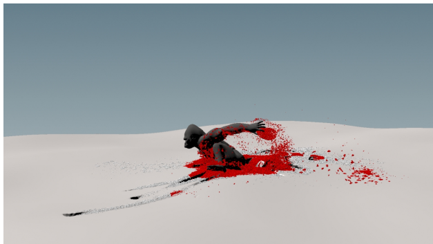
Fig. 13 Only active snow particles (in red), in the areas around dynamic objects and moving particles, are computed in our examples. This considerably lowers computation times.
