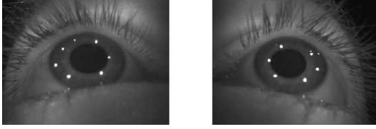
Figure 3: Corneal reflections of infrared emitting diodes
