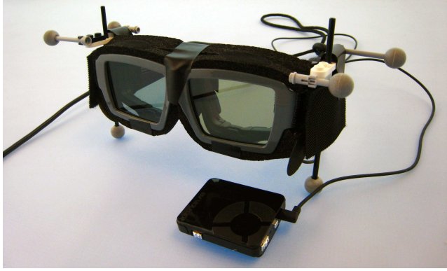
Figure 4: Eye Tracking Glasses combined with Volfoni active stereoscopic glasses. The markers are placed on the ETG so that head's and ETG's reference frames match, allowing us to collect sight directions in local (ETG) and global (CAVE room) coordinate systems
