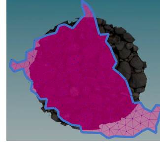
Figure 5: Example of a patch mesh in uv domain, where the boundary ( B_V = 0 ) is shown as the blue line around the patch.
