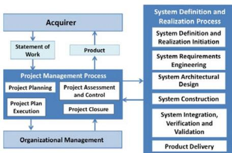
Figure 3: Processes of the Systems Engineering Basic Profile
